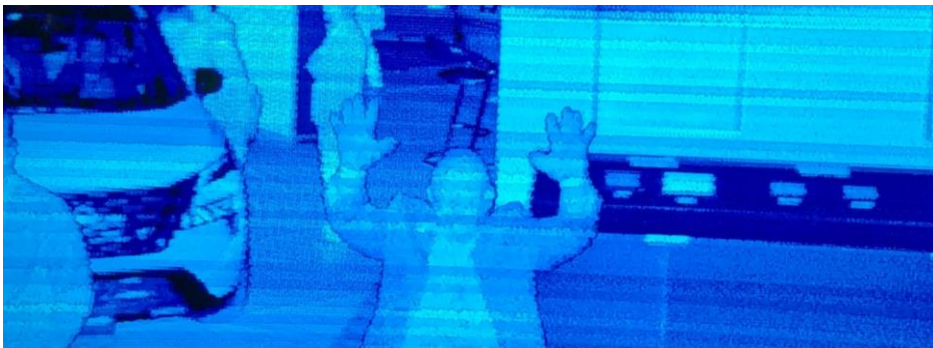
Innoviz Two lidar with 0.05° resolution can distinguish between fingers
