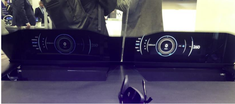
Normal HUD (Left) and AGC glass solution for HUD (Right)
