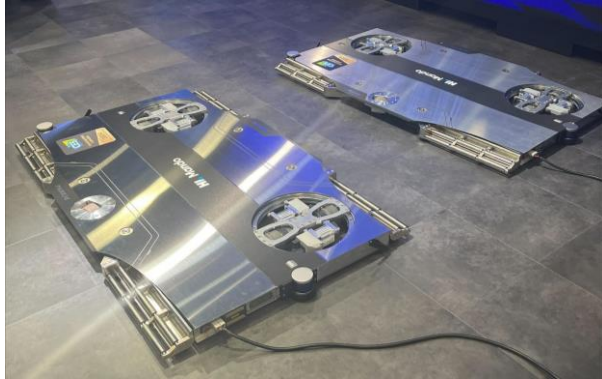
HL Mando Parkie robot that can lift vehicle by tired and move it autonomously
