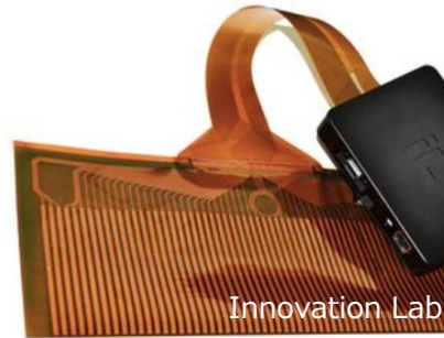
Battery cell pressure sensor
