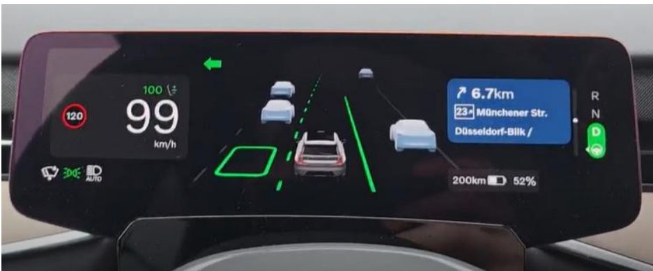
Once AD is activated the lane markings become green and automatic lane change is available
