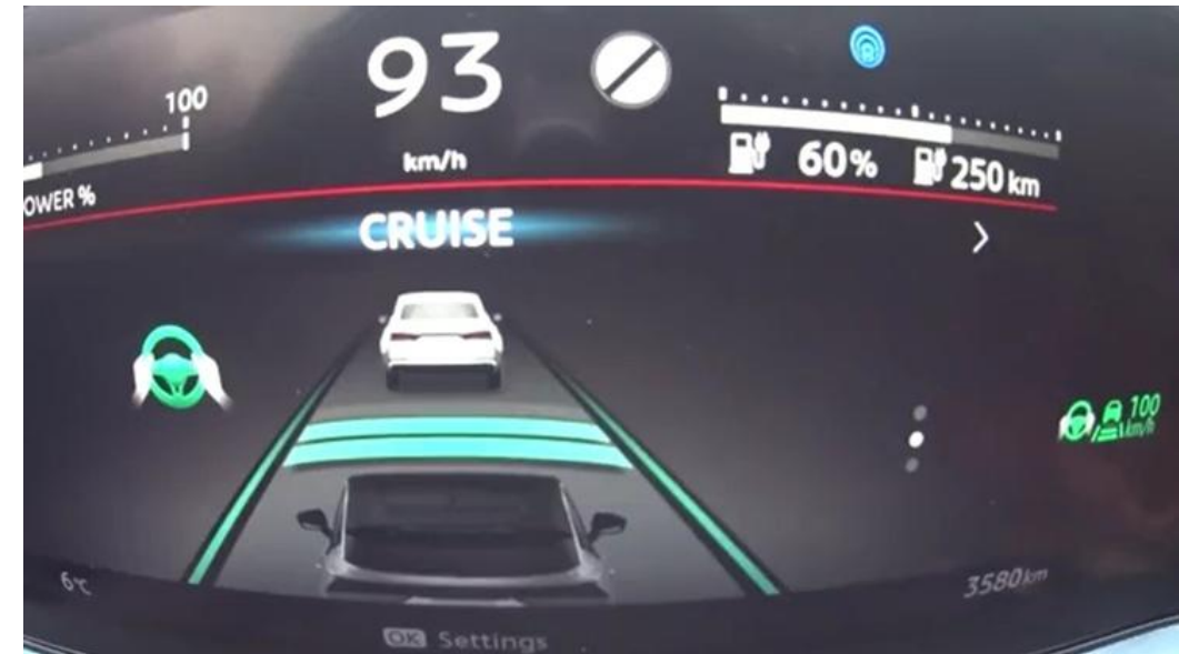
Unlike the Nissan Ariya, Volvo simplifies the experience by eliminating the separate Cruise Control and headway selection features
